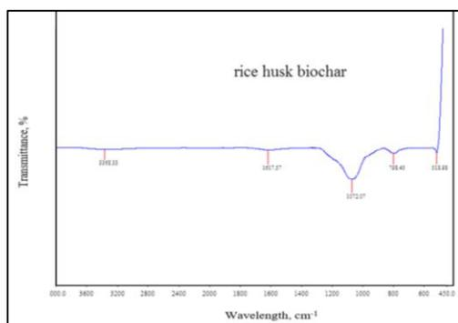
Figure 1 FTIR - Spectrum of RHB used in this study.
